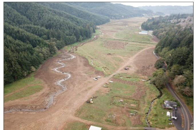
Newly re-meandered channel in the mainstem of Kentuck Creek.
